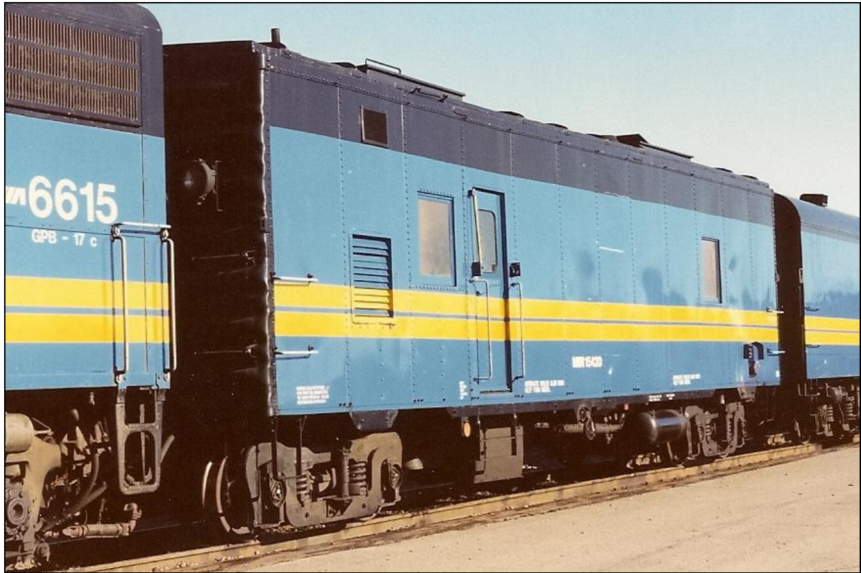
VIA Steam Generator Unit No. 15420
