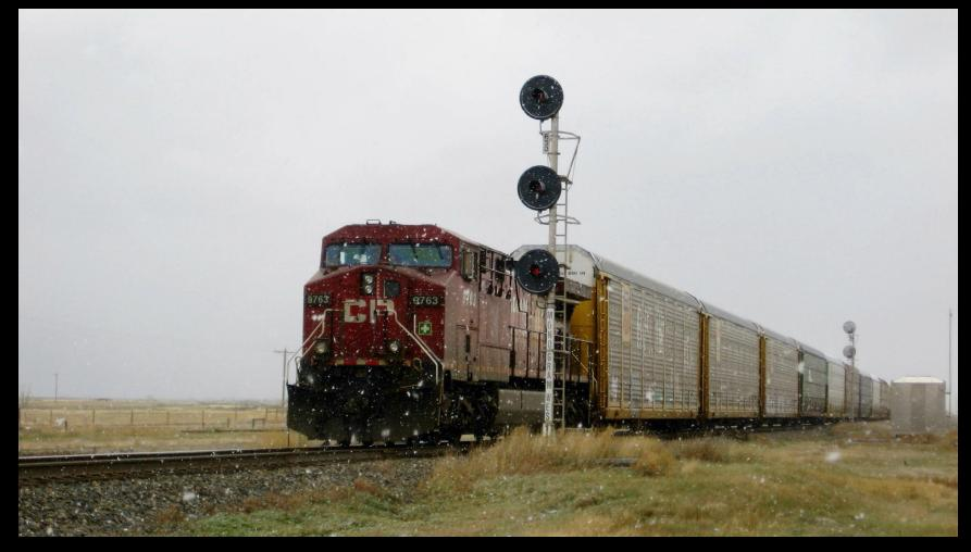
CPR 9763 is the rear Distributed Power Unit on 128 platform IMS 9705 EAST as it passes the signals in the snow at Monogram West, M 63.0 Brooks Sub., on 10 Oct 2009. Monogram is a 7,701 foot long passing siding about 500 feet east of where the CPR main line crosses the Brooks Aqueduct. Monogram has never had a station or grain elevators; these were at Brooks, 4 miles west at M 66.8.
